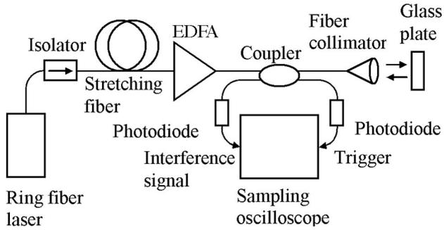
Fig. 1. Schematic representation of the measurement setup. EDFA, erbium-doped fiber amplifier.
