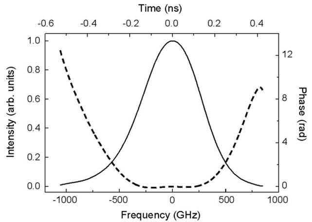
Fig. 4. Spectral intensity  $I(\omega)$  (solid curve) and spectral phase  $\varphi(\omega)$  (dashed curve) of the input pulse, reconstructed from Fig. 3. The time and frequency scales are related by Eq. (2).
