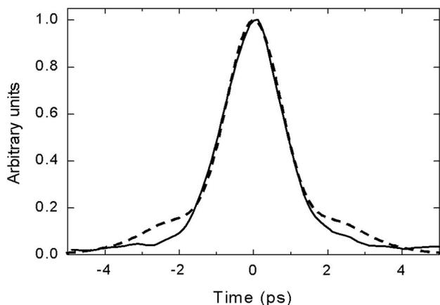
Fig. 7. Autocorrelation of the laser pulse, measured (solid curve) and calculated (dashed curve) for the reconstructed pulse intensity shown in Fig. 5.
