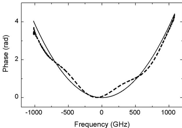
Fig. 6. Measurements of the phase response of a 9 m long conventional fiber obtained by our method (dashed curve) as well as by measuring the frequency dependence of the group delay (solid curve).
