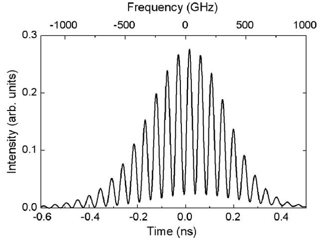
Fig. 2. Oscilloscope trace of the interference between two replicas of the stretched pulse reflected from the two surfaces of a glass plate. The time and frequency scales are related by Eq. (2).
