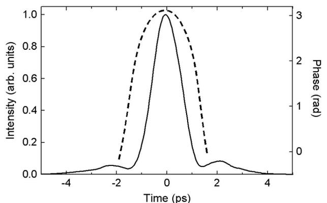
Fig. 5. Reconstructed temporal intensity  $I(t)$  (solid curve) and phase  $\varphi(t)$  (dashed curve) of the fiber laser pulse.
