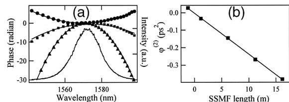
Fig. 3. (a) Measured spectral intensity (solid curve) and phase induced by removing 1.2 m (circles) and adding 1.2 m (squares) and 6.2 m (triangles) of SSMF. The expected parabolic spectral phases calculated with  $D = 18 \text{ ps/nm/km}$  are also plotted. (b) Second-order dispersion  $\varphi^{(2)}$  versus the SSMF length.
