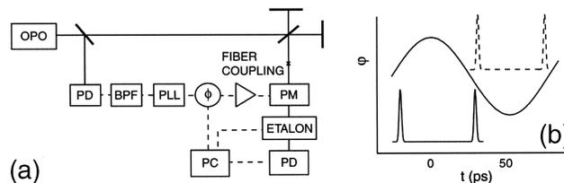
Fig. 1. (a) Schematic of the experimental setup: PDs, photodiodes; BPF, bandpass filter;  $\phi$ , phase shifter; PM, phase modulator. Optical paths are plotted as a continuous line, electrical connections are plotted as a dashed line. (b) Two different timing alignments between the optical pulses and the 10-GHz drive of the phase modulator.
