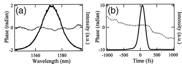
Fig. 2. (a) Spectral phase (dashed curve) and intensity (solid curve) and (b) temporal phase (dashed curve) and intensity (solid curve) of the OPO pulses.
