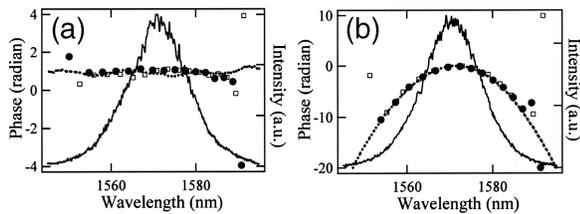
Fig. 4. (a) Spectral intensity (solid curve) and phase of the initial pulse for 100 (dashed curve), 20 (squares), and 5  $\mu\text{W}$  (circles) of power. (b) Spectral intensity (solid curve) and phase of the pulse after propagation in 5 m of SSMF for 160 (dashed curve), 20 (squares), and 5  $\mu\text{W}$  (circles) of power. Spectral intensities are plotted for only the highest powers for clarity.
