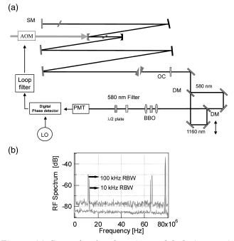
Fig. 3. (a) Setup for  $f_{ceo}$  detection and lock (see text). SM, silver mirror; DM, dichroic mirror; LO, local oscilator. (b) Measured carrier-envelope beat signal from the 80-MHz laser with 10- and 100-kHz resolution bandwidths (RBW).
