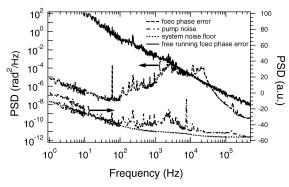
Fig. 4. Spectral densities of the phase error signal at the output of the digital phase detector for the  $f_{ceo}$  lock (dashed curve) and free-running  $f_{ceo}$  (solid curve), with the scale on the left. Spectral density of the pump noise recorded in the absence of  $f_{ceo}$  feedback (dashed-dotted curve) and system noise floor (dotted curve), with the scale on the right. The major contribution to  $f_{ceo}$  noise is due to pump noise. PSD, phase error spectral density.
