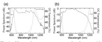
Fig. 2. Measured output spectrum for lasers with (a) 80-MHz repetition rate and (b) 150-MHz repetition rate. In both cases the octave is reached at  $\sim 25$  dB below the average power level. The average mode-locked power is 90 mW for both lasers. Also shown (dotted curves) are the respective OC transmission curves for (a) the ZnSe/MgF<sub>2</sub> Bragg stack and (b) a broadband SiO<sub>2</sub>/TiO<sub>2</sub> stack. Both have  $\sim 1\%$  transmission at 800 nm.
