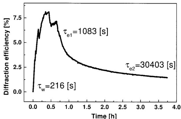
Fig. 2. Recording and readout curve for a plane-wave hologram in a 90-deg-cut LiNbO<sub>3</sub> crystal doped with 0.15-wt. % Fe<sub>2</sub>O<sub>3</sub> and 0.015-wt. % MnO. The recording beams are from a solid-state green laser (wavelength 532 nm, ordinary polarization,  $1/e^2$  beam diameter 2.0 mm, and intensity 80 (mW/cm<sup>2</sup>/beam). The sensitizing light is from a laser diode (Nichia, wavelength 401 nm, linearly polarized, intensity 20 mW/cm<sup>2</sup>).
