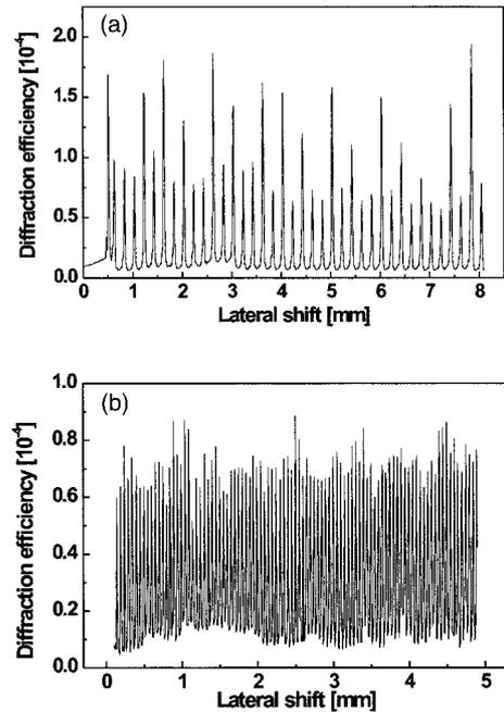
Fig. 5. (a) Spatial multiplexing of 40 localized holograms. (b) Spatial multiplexing of 100 localized holograms.
