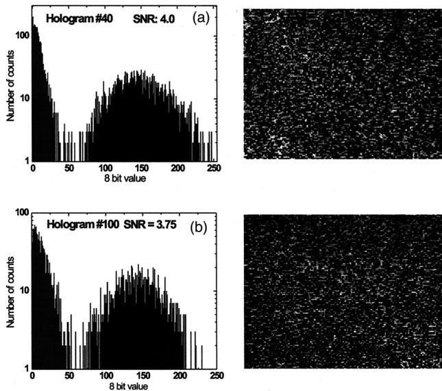
Fig. 6. (a) Sample reconstructions and SNR values from the experiment with 40 holograms. (b) Sample reconstructions and SNR values from the experiment with 100 holograms.
