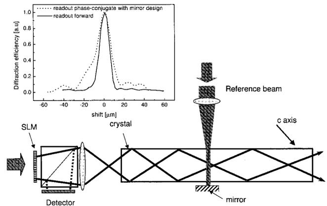
Fig. 10. Compact module by use of a mirror for phase conjugation. Also shown is the spatial selectivity of the forward and conjugate reconstruction.
