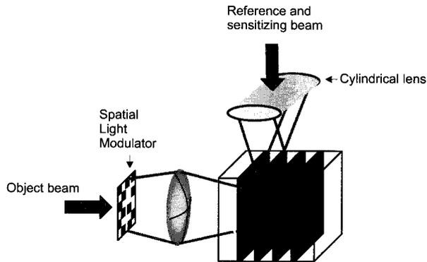
Fig. 1. Localized recording in doubly doped LiNbO<sub>3</sub>.
