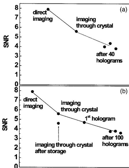
Fig. 7. SNR comparison with a focused reference beam of spot size (a) 100  $\mu\text{m}$  and (b) 25  $\mu\text{m}$ .
