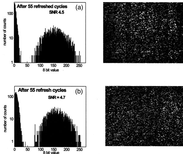
Fig. 9. Histogram and reconstruction of the central hologram before and after the refresh cycle: (a) 100- $\mu\text{m}$  focus, (b) 25- $\mu\text{m}$  focus.
