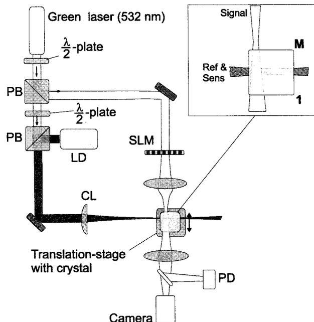
Fig. 3. Recording setup for the SNR measurement. LD, laser diode; CL, cylindrical lens; PD, photodiode; PB, polarizing beam splitter.
