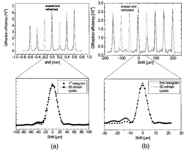
Fig. 8. Diffraction efficiency versus position before and after 55 refresh cycles of the central hologram: (a) 100- $\mu\text{m}$  reference focus, (b) 25- $\mu\text{m}$  reference focus.
