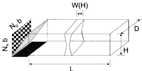
Fig. 12. Memory capacity for the phase-conjugate module.
