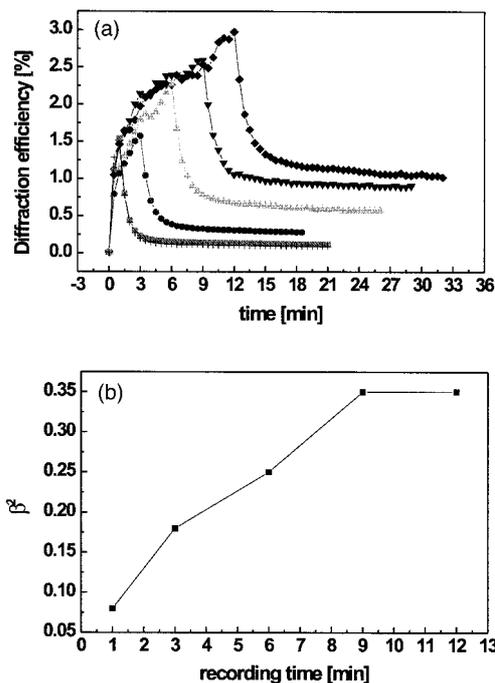
Fig. 4. (a) Recording curves with a focused green 532-nm reference at 35  $\mu\text{m}$  ( $1/e^2$  value) and erasing with reference beam only. (b) Persistence  $\beta^2$  as a function of recording time.
