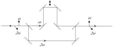
Figure 3.7: A traditional delay line consisting of beamsplitters and mirrors.
