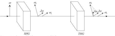
Figure 3.3: Simple THG with type 2 SHG.
