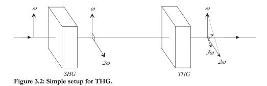
This setup works very well and is easy to align. The previous setup in the lab used this layout. However the efficiency is limited by several things. The most obvious one is that the polarizations are wrong. And the group velocity difference makes the temporal overlap in the THG crystal less than perfect. This is covered in section 3.1.2.
