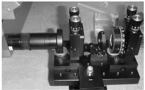
Picture 6.1: Photograph of the finished tripler.
