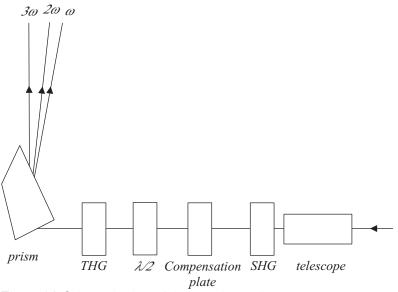
Figure 4.1: Schematic view of the experimental setup.
