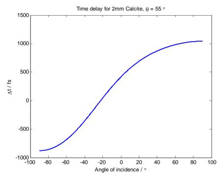
Figure 3.14: Example curve for a Calcite compensation plate.
