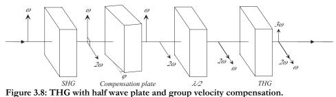
The behavior of the extraordinary wave is fairly complex due to the walk off. In negative crystals the extraordinary wave bends way from the optical axis. This is a simple example with normal incidence.
