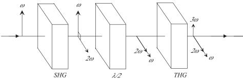
Figure 3.4: THG with half wave plate to correct the polarization.
