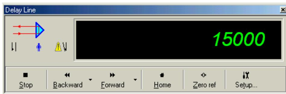
Fig. 37. Delay line stopped by limit switch.
