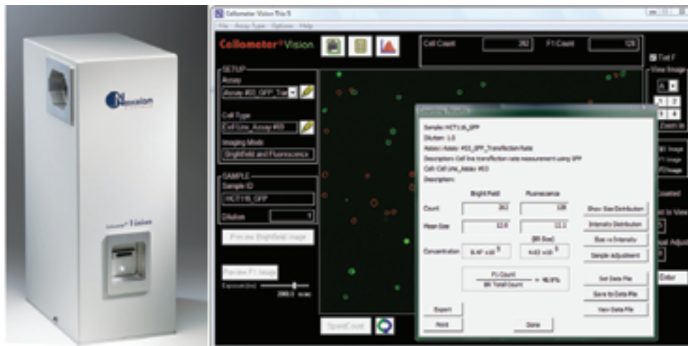
Figure 1 The Cellometer Vision brightfield/fluorescence imaging system consists of a compact instrument and image analysis software. Cell images, counting results, and other data are displayed on-screen.
