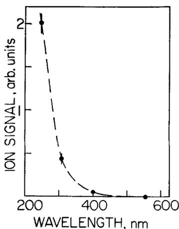
Fig. 5. Efficiency of laser stimulated desorption at various radiation wavelengths
