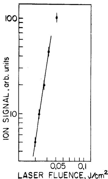
Fig. 4. Laser-stimulated ion signal as a function of the laser fluence incident on the tip. Field strength at the tip  $0.36$  V/Å, radiation wavelength  $555$  nm
