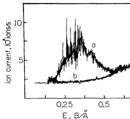
Fig. 2. Ion current as a function of the field strength at the tip, the field strength being increased in a linear fashion
