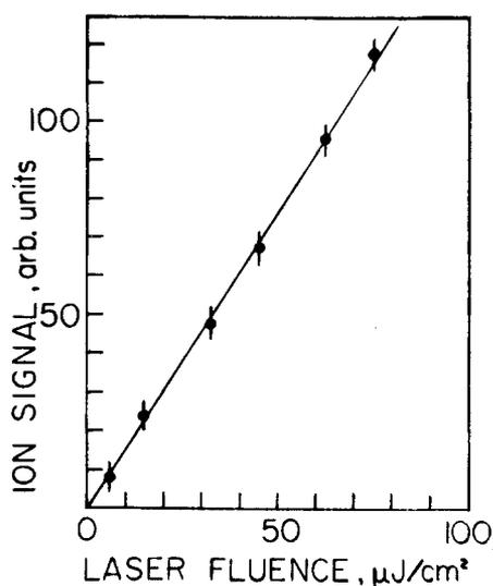
Fig. 3. Laser-stimulated ion signal as a function of the laser fluence incident upon the tip. Field strength at the tip  $0.36$  V/Å, radiation wavelength  $308$  nm
