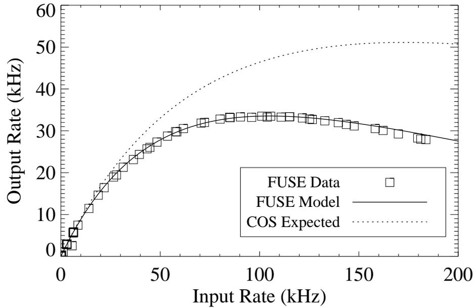
Figure 4. A comparison of the measured FUSE digitizer livetime vs. the expected livetime of the COS design. The livetime at 100 kHz will increase from 33% to 47%.
