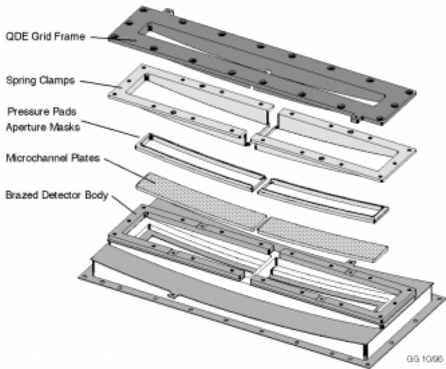
Figure 1. Exploded view of the COS FUV detector. The two MCP stacks are 95 mm by 20 mm.
