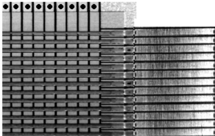
Figure 2. Top right corner of a prototype COS anode. The wide vertical traces are the Cu helical delay line that senses the X position of an MCP event. The narrow horizontal traces on the left are the Y “fingers” that collect ~35% of the event charge and inject it into the small Y helical delay line on the right. The pattern period in the X direction is 0.63 mm.
