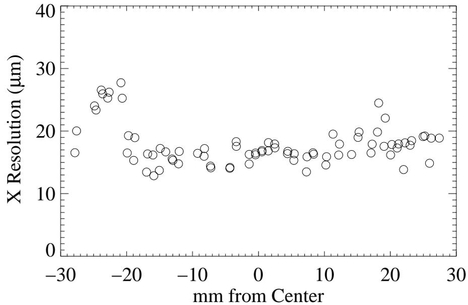
Figure 3. Measurement of spatial resolution in the X direction (FWHM) as a function of X position using the COS prototype anode. The pinhole mask used to define the UV input had 10  $\mu\text{m}$  holes. The COS requirement is 25  $\mu\text{m}$  FWHM.
