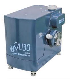
The MSA-130 is a high-aperture double monochromator with the focal length of 130 mm, which operates in the modes of both addition and subtraction of dispersions. The monochromator operation modes are changed by switching of a selector knob from the position "Addition" to "Subtraction" and vice versa.
