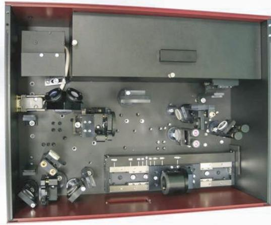
Cross-correlator includes opto-mechanical assembly and electronics with USB interface. System is easy to operate and includes a full set of user friendly software tools for data collection and analysis.
