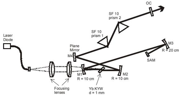
Fig. 2. Experimental set-up for the mode-locked Yb:KYW laser. M1 – M3, curved mirrors; R, radius of curvature; M4, high-reflective plane mirror; OC, output coupler with different transmissions; SAM, saturable absorber mirror.
