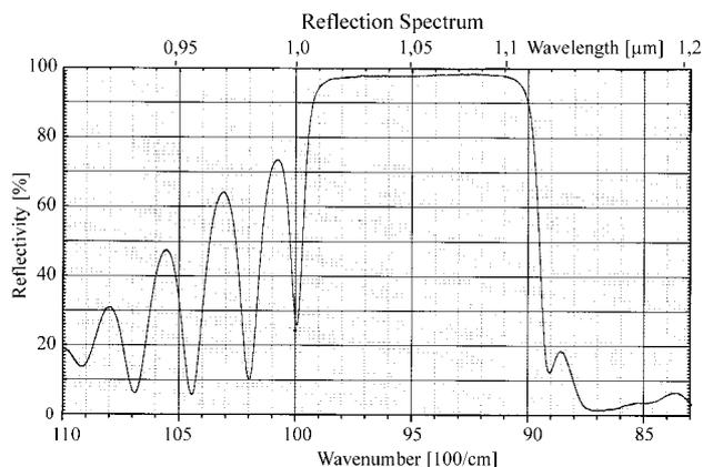
Fig.1. Spectral reflection of unsaturated SAM with 1.2% modulation depth.
