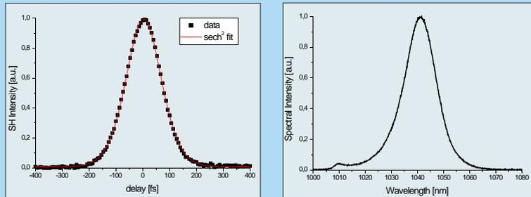
The autocorrelation trace (left) and the corresponding optical spectrum (right) of the shortest pulses delivered from the Yb:KYW laser. They were obtained using a 2% modulation depth saturable absorber and a 1% transmission output coupler. The red line shows the theoretical curve assuming a pulsewidth of 100-fs and a  $sech^2$  - pulse shape. The spectrum is centered at 1041 nm and has a bandwidth of 14.2 nm FWHM. The output power was 52 mW at a pump power of 4.4 W.
