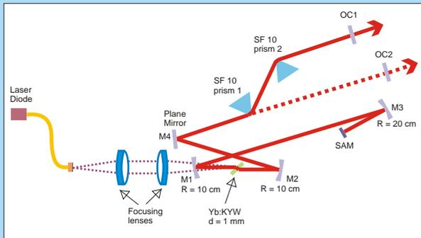
M1-M3, curved mirrors; R, radius of curvature; M4, high-reflective plane mirror;
