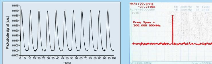
The pulse train was recorded with a silicon photodiode with a rise time of 2 ns and a 500 MHz - oscilloscope. The frequency spectrum does not show bandsides.
