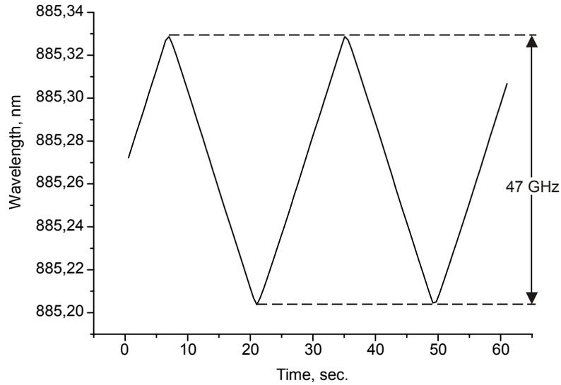
Fig. 6. Automatic smooth scanning of Ti:Sapphire laser frequency in the free-running generation mode (regime of passive frequency stabilisation).
