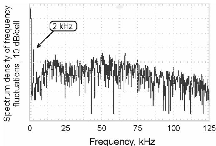
Fig. 5. Spectral density of the frequency noise of the stabilized laser in Dye configuration, linewidth: 75 kHz rms.
