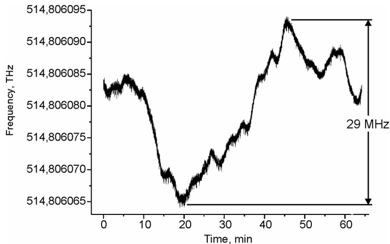
Fig. 4. Dependence of laser frequency on time obtained with wavelength meter WS/Ulimate.
