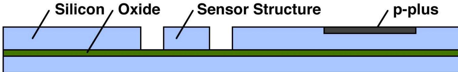
Start with a “generic” MEMS device made from silicon, prior to being released from the substrate by HF. Silicon layer may be single crystal (SOI), or poly-si (Bosch epi-poly structural material, for example).
