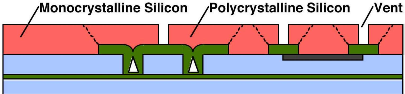
**Deposit Thick Epi-Poly. This forms poly where grown over LTO, and forms single-crystal Si where grown over single-crystal Si.**
