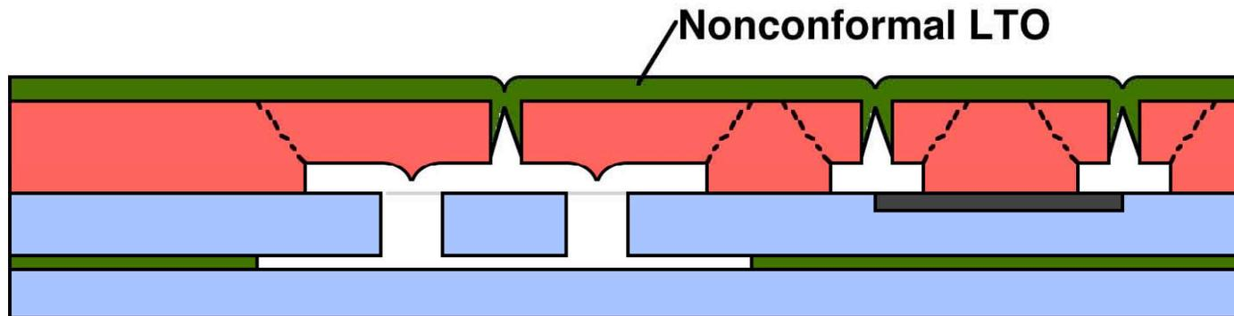
The encapsulation oxide is removed in a Vapor HF etcher, developed by Bosch (Prototype installed at Stanford), and the device is sealed by a second non-conformal LTO. TEOS and other thick oxide processes being explored
