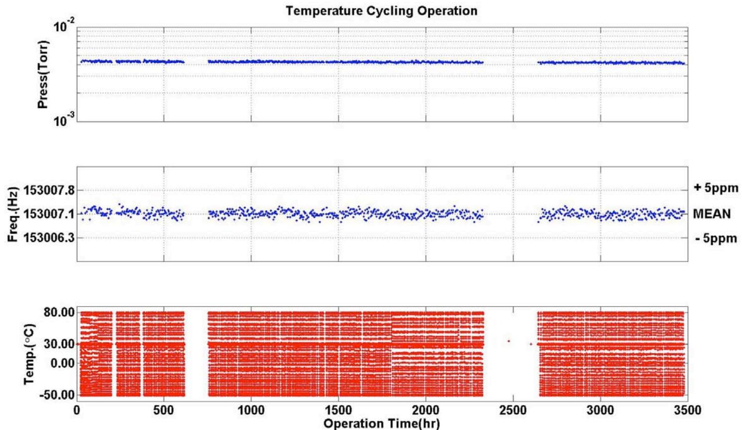
As with fixed-temperature tests - no evidence for leakage through encapsulation.
