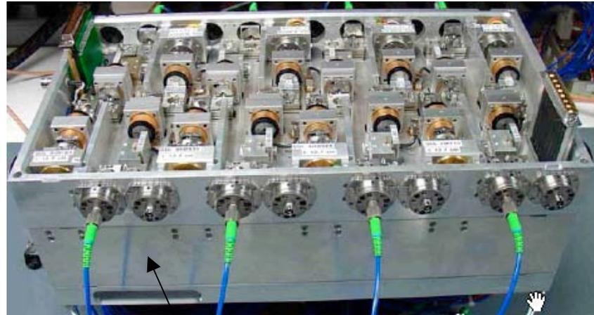
**Laser and control electronics, supports multiple (4 to 6) sensor heads.**
