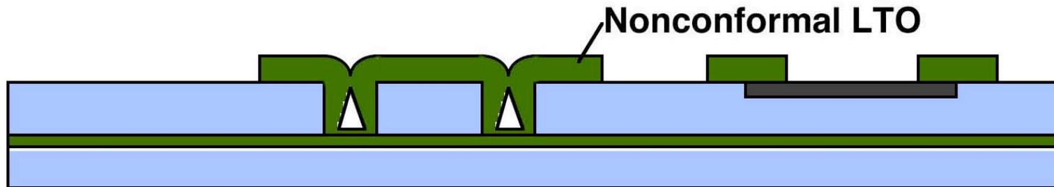
Deposit a thick (3-5  $\mu\text{m}$ ) non-conformal Low-Temperature oxide. This oxide fills and seals structures around the device, producing a complete sacrificial encapsulation.
