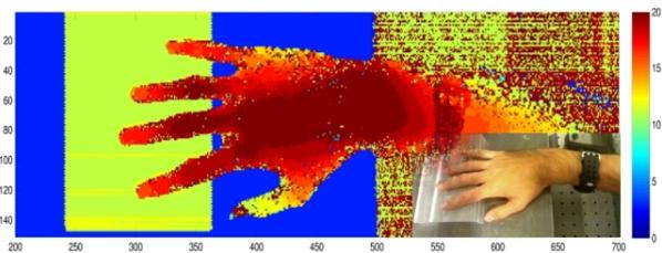
**Fig. 4** 300 GHz FMCW-ranging image of a hand
