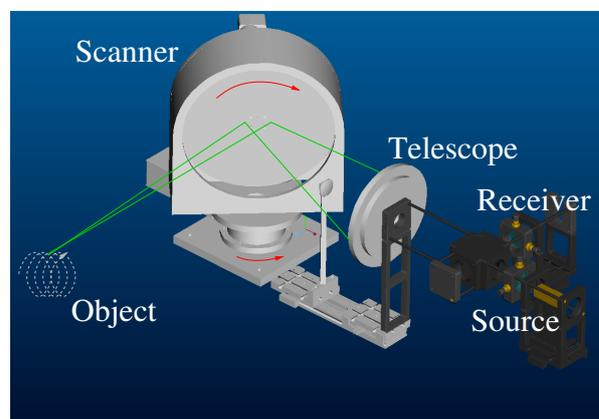
Fig. 1 3D CAD drawing of the single-pixel scanner setup
