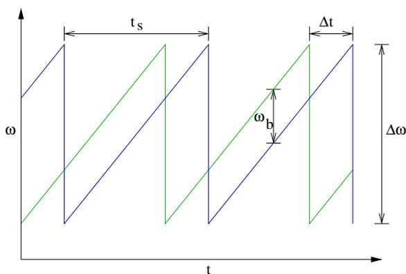
**Fig. 3** Illustration of FMCW ranging by sawtooth sweeping
