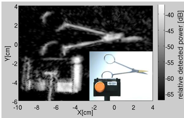
**Fig. 2** 620 GHz image of the scissors shown in the inset
