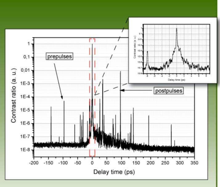
Cross-correlation measurements of a regenerative amplifier taken over a range of 550 ps show pre-pulses, post-pulses, and the main pulse relative to the ASE level. A 16 ps scan of the main peaks (inset) shows further temporal structure of the main peak. The relative strength of the secondary peaks is easily seen at both ranges.
